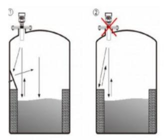
The transducer end must at least protrude 10mm out of socket.
